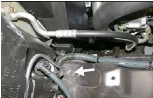
11. Remove the hex bolt located directly below the windshield washer reservoir as shown.
