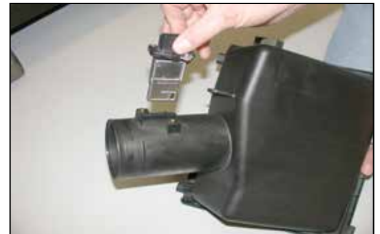
25. Remove the mass air sensor from the air cleaner cover as shown.
